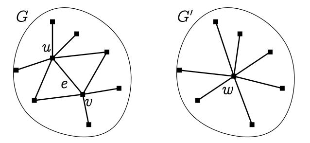
When edges are contracted, a planar graph remains planar.
