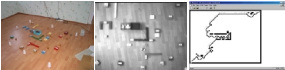
Figure 3. The test environment (to the left), the same environment seen through the overview camera (in the middle) and as modeled by the control program (to the right).
