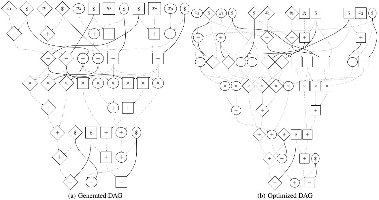
Figure 4: Multiplication protocol circuit
