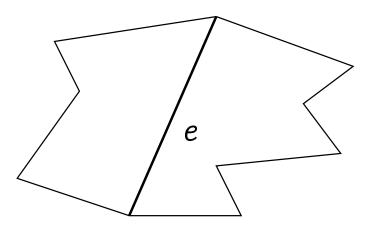
The graph G - e has one edge and one face less than the graph G. According to the induction hypothesis, we have n + (f-1) - (m-1) = 2. This implies n + f - m = 2.
