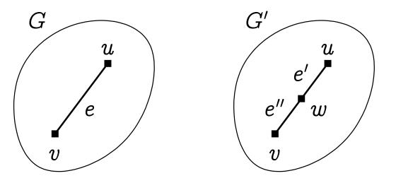
The edge e is replaced by a the vertex w and edges e', e''.
